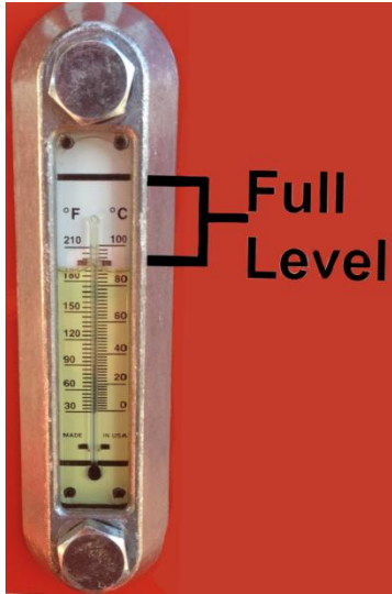
Fig. 5-2 Hydraulic Fluid Level and Temp. Gauge
