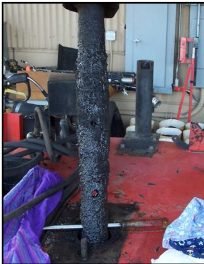
Fig. 6-6 Supporting the Agitator Away from the Material Pump
