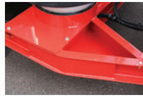
Webbed Reinforced Welded Frame
