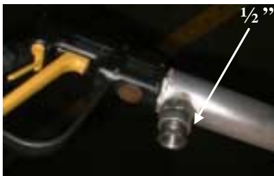
Wand hose connector with the supplied bushing. If you purchase the new high flow wand the bushing will connect to the old hose.
