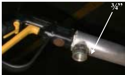
The new SuperShot wand/hose 3/4" connector. This is for the high flow hose.
